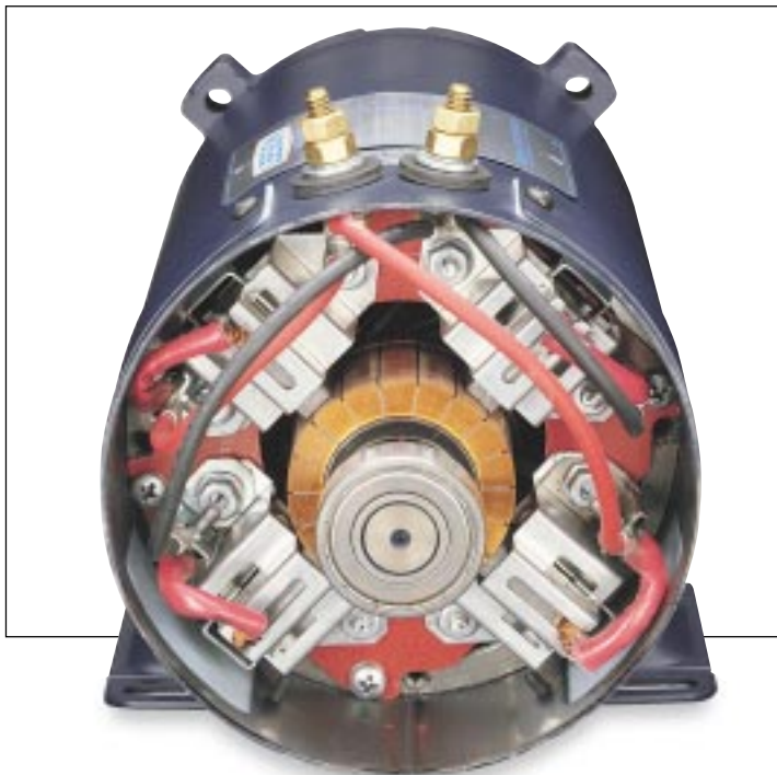
IEC and NEMA frame DC motors from LEESON feature oversized brushes, accessible without disassembly of the motor. Integral constant pressure springs and bi-directional brush holders help ensure long service before maintenance — up to four times that of other DC motors. Four brushes are used in larger horsepower low voltage motors.
