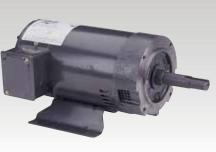
Lincoln has a full line of Signature Series pump motors for a variety of fluid handling applications. Choose from TEFC or ODP, close-coupled JM and JP or Jet Pump mounting, single or three phase. All have premium insulation systems for long life, high quality ball bearings, easy-to-read nameplates and phosphate coated shafts. Jet Pump motors include automatic reset thermal overload protection. All Signature Series pump motors are made in the U.S.A.
