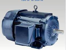
Crusher Duty motors are designed for severe belted-load applications. They are available in cast iron or steel construction and include a drive-end roller bearing, a high-strength steel shaft, Class F thermostats, high starting torque, and PWS/YDS capability.
