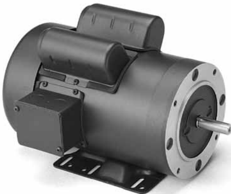
On industrial duty motors, capacitors are usually protected by metal cases attached to the motor frame. This capacitor start/capacitor run motor has two cases.
