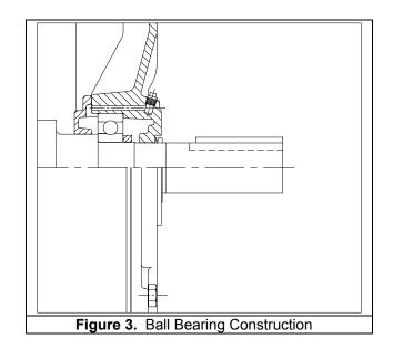
Protect the shaft end with a cap. If bearing is reusable, make certain the puller applies pressure against the bearing inner race only. If puller will not hook the bearing inner race, fabricate a split bushing and install it between the bearing and the puller hooks.
