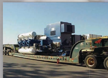
4000 HP Medium Voltage Motor & Reciprocating Ariel Compressor Unit Being Transported
