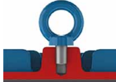
Figure 4-2 – Incorrect tightening of the eyebolt
