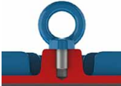
Figure 4-1 – Correct tightening of the eyebolt
