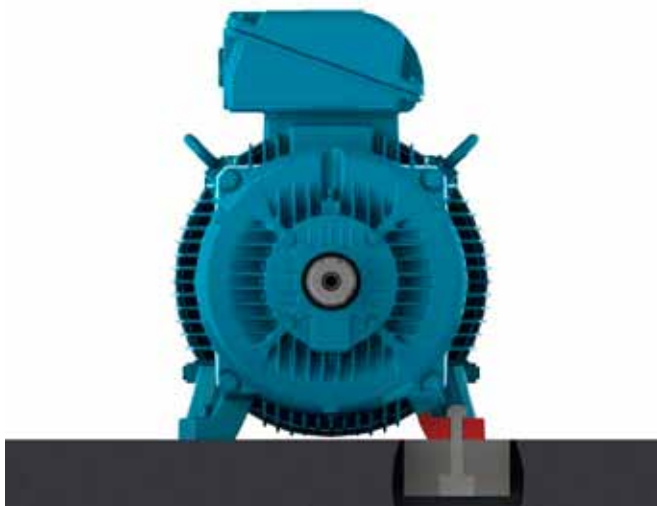
Figure 6-3 – Motor installed on concrete base
